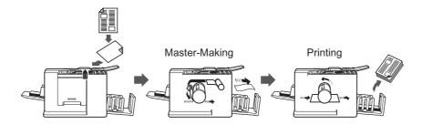
An original placed on the ADF unit is scanned by the scanner, and a generated master is rolled around the Print Drum (Cylinder).
