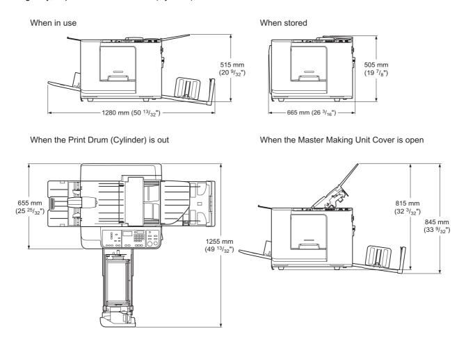
• The distance from the right side of the machine to the right edge of the stand (desk, etc.) should be 10 cm (3 15/16") or less. If the distance is greater than 10 cm (3 15/16"), the stand will interfere with the Paper Receiving Tray and it will not be possible to set the tray up correctly.
