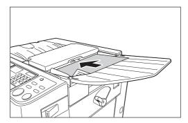
The bottom original is scanned first.
