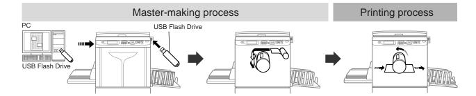
Output the data created on a computer to the USB Flash Drive and connect the USB Flash Drive to the USB slot. The generated master is rolled around the Print Drum (Cylinder).
