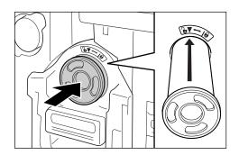
Align the arrow on the Ink Cartridge to the  $\mathbf{\nabla}$  mark on the drum (cylinder) unit, and insert until it stops.
