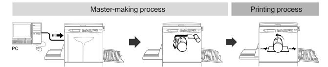
Data sent from a computer is transformed into images, and a generated master is rolled around the Print Drum (Cylinder).
