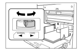
Position the Paper Feed Pressure Adjustment Lever according to the finish of the paper.
