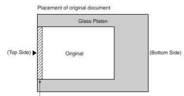
Top: This area (5mm (<sup>3</sup>/<sub>16</sub>") from the top edge) cannot be scanned.
