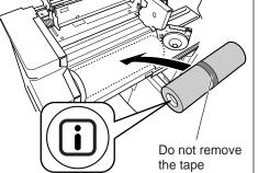
Remove the plastic shrink wrap from the new Master Roll, and place in with the I mark to the left.
