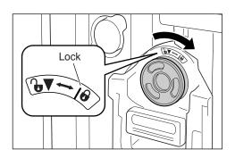
Turn the lnk Cartridge clockwise (  $\textcircled{\phantom{a}}$  ) and lock in position.
