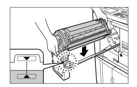
Align the  $\checkmark$  mark on the Print Drum (Cylinder) with the  $\blacktriangle$  mark on the guide, and place the Print Drum (Cylinder) horizontally onto the rail.
