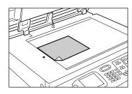
Place the original face down on the Glass Platen. Align center on the top edge, and close the Platen Cover.
