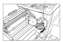
**6** Remove the depleted Master core.
