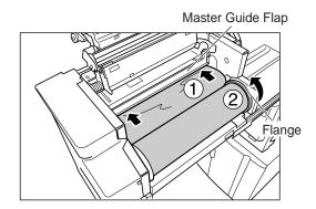
Insert the leading edge of the master into its entrance under the Master Guide Flap and advance it as far in as it will go ( $\bigcirc$ ). If the Master is loose, turn the flange at the right towards the rear and rewind ( $\bigcirc$ ).
