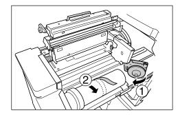
Remove the tape once the Master Roll Holder has been closed.
