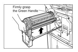
Use both hands to lift the Print Drum (Cylinder) straight up to remove from the rail. Proceed with replacing the drum (cylinder), removing the paper jam, etc..
