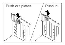
Alignment of paper is affected by sizes and strength of paper. Adjust the Paper Arrangers so that printed paper is aligned.
