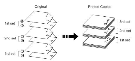
Refers to an original produced with () for Print Drum (Cylinder) 1, and (2) for Print Drum (Cylinder) 2.
