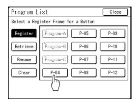
Unused buttons are displayed with a solid line. Used buttons are grayed out and are not available.
