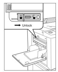
Grasp the Master Disposal Box handle and pull the box forward.
