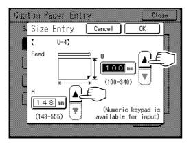
Facing the paper feeding direction (into Paper Feed Tray), enter W (width) and H (height). Touch either  $[ \bullet ] [ v ]$ , or use Print Quantity Keys.
