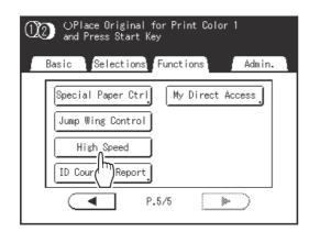
"High Speed" is set and the Print Speed indicator on the control panel turns off.
