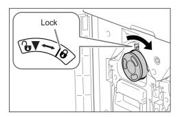
Turn the lnk Cartridge clockwise (  $\bigodot$  ) and lock in position.
