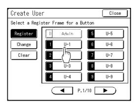
Unused buttons are displayed with a solid line. Used buttons are grayed out and are not available. (Another user has been registered.)
