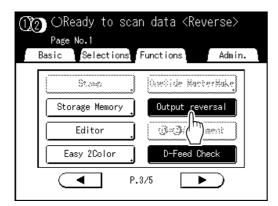
The button is highlighted and "Output reversal" is set to "ON".
