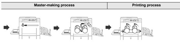
Place the second original. A placed original is scanned by the scanner, and a generated master is rolled around the Print Drum (Cylinder) 2. After a while, proof copy with Dual-Color printing is printed. After checking the print result, enter the number of copies to be printed and start printing.
