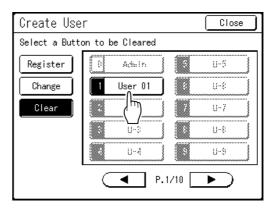
Registered buttons are displayed with a solid line. Unregistered buttons and "0 Admin" button are grayed out and are not available.
