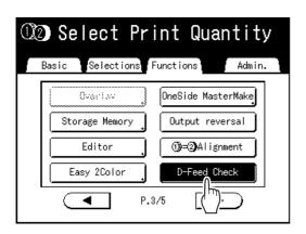
The button changes from being highlighted (b/w) to the normal display, and "D-Feed Check" is set to "OFF".
