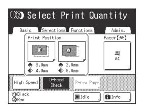
Adjusting the Print Position of Both Print Drums (Cylinders) Together
