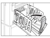
**2)** Pull up the Paper Arrangers, slide the Receiving Tray Paper Guides to the left and right as far as they will move and fold in.
