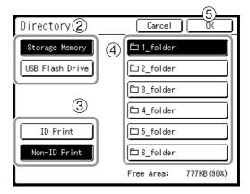
If the USB Flash Drive is not connected, **[USB Flash Drive]** is grayed out and not available.
