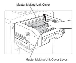
Grasp the Master Making Unit Cover Lever and open the Master Making Unit Cover.
