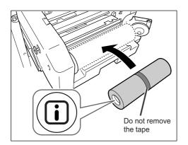
Remove the plastic shrink wrap from the new Master Roll, and place in with the **I** mark to the left.
