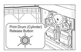
If the indicator is off, press the Print Drum (Cylinder) Release Button to turn it on.
