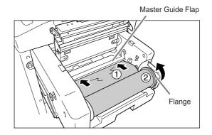
Insert the leading edge until it stops  $(\bigcirc)$ . If the master is loose, turn the flange at the right inward to rewind  $(\bigcirc)$ .
