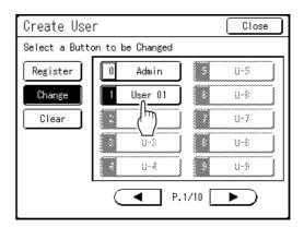
Registered buttons are displayed with a solid line. Unregistered buttons are grayed out and are not available.
