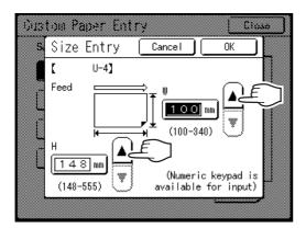
Facing towards the paper feeding direction (into Paper Feed Tray), enter W (width) and H (height).
