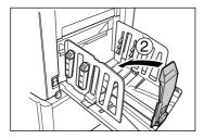
2) Pull up the Paper Arrangers, slide the Receiving Tray Paper Guides to the left and right as far as they will go and fold in.
