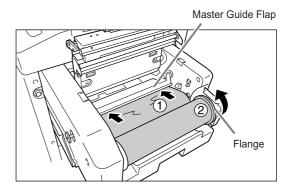
Insert the leading edge until it stops (1). If the master is loose, turn the flange at the right inward to rewind (2).
