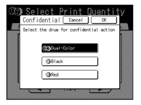
♦ When only one Print Drum (Cylinder) is set in the machine
