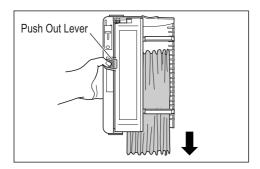
Tilt the Master Disposal Box forward and directly discard the used master into the garbage box (or bag) by grasping the Push Out Lever.
