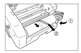
Remove the tape once the Master Roll Holder has been closed.
