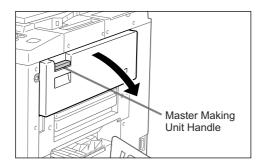
Grasp the Master Making Unit Handle and pull out to open.
