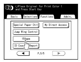
"150 ppm" is set and the Print Speed indicator on the control panel turns off.
