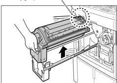
Use both hands to lift the Print Drum (Cylinder) straight up to remove from the rail. Proceed with replacing the Print Drum (Cylinder), removing the paper jam, etc..
