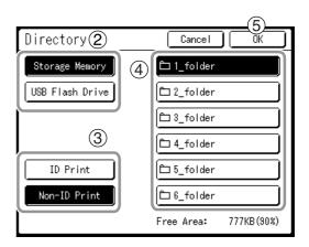
If the USB Flash Drive is not connected, [USB Flash Drive] is grayed-out and is not available.
