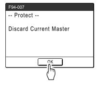
Touch [OK] to discard the master remaining on the Print Drum (Cylinder).
