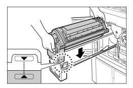
Align the ▼ mark on the Print Drum (Cylinder) with the **\( \Lambda \)** mark on the guide, and place the Print Drum (Cylinder) horizontally onto the guide.
