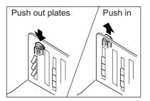
Alignment of paper is affected by sizes and strength of paper. Adjust the Paper Arrangers so that printed paper is aligned. Press the Paper Arranger to push the plates out, pull up to pull them in.
