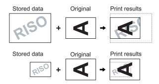
The stored data is overlaid after being centered at the top of the original. You cannot adjust the overlay position.
