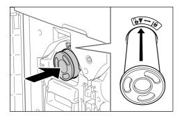
Align the arrow on the Ink Cartridge to the mark on the Print Drum (Cylinder) unit, and insert until it stops.
