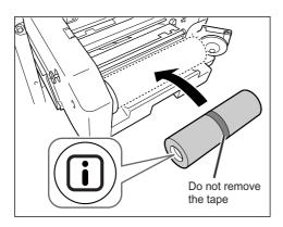
Remove the plastic shrink wrap from the new Master Roll, and place in with the T mark to the left.
