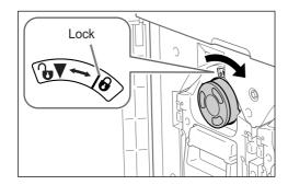
Turn the Ink Cartridge clockwise ( ) and lock in position.
