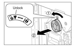
Turn the Ink Cartridge to the counter clockwise ( and then pull it out.
