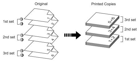
Refers to an original produced with (f) for Print Drum (Cylinder) 1, and (2) for Print Drum (Cylinder) 2.
