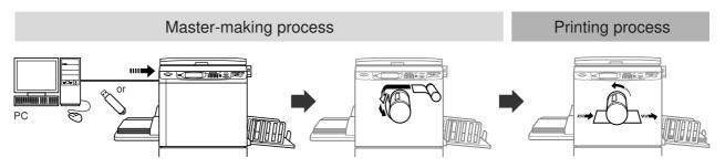
Transfer the original data created with a computer to the machine via a network or USB Flash Drive. A generated master is rolled around the Print Drum (Cylinder).
