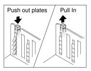
Alignment of paper is affected by sizes and strength of paper. Adjust the Paper Arrangers so that printed paper is aligned.
