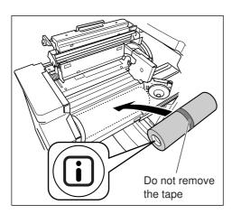
Remove the plastic shrink wrap from the new Master Roll, and place in with the I mark to the left.
