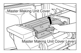
Grasp the Master Making Unit Cover Lever and open the Master Making Unit Cover.
