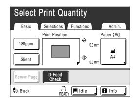
When a proof copy is printed, the Print Basic Screen will be displayed automatically. Check the proof copy; e.g., print position and density.
