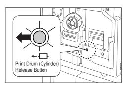
If the indicator is off, press the Print Drum (Cylinder) Release Button to turn it on.
