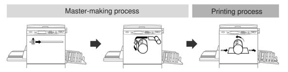
A placed original is scanned by the scanner, and a generated master is rolled around the Print Drum (Cylinder). After a while, proof copy is performed. After checking the print result, enter the number of copies to be printed and start printing.
