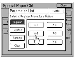
Unused buttons are displayed with a solid line. Used buttons are grayed-out and are not available.
