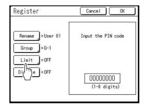
2 Touch the limit input box and enter the upper limit number using the Print Quantity Keys.
