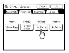
If the button has a function already assigned to it, the newly selected function will overwrite the previous function.
