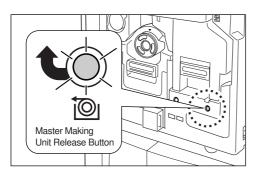
If the indicator is off, press the Master Making Unit Release Button to turn it on.
