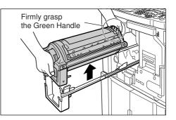
Use both hands to lift the Print Drum (Cylinder) straight up to remove from the rail. Proceed with replacing the Print Drum (Cylinder), removing the paper jam, etc..
