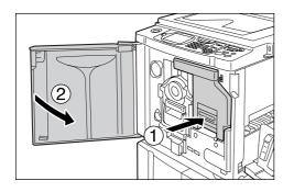
Return the Master Making Unit to its original position and close the Front Cover.
