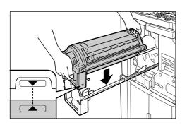
Align the  $\checkmark$  mark on the Print Drum (Cylinder) with the  $\blacktriangle$  mark on the guide, and place the Print Drum (Cylinder) horizontally onto the guide.
