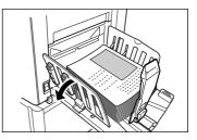
For the machine equipped with the Auto-control Stacking Tray, press the Receiving Tray Paper Guides' Opening Button and remove the paper.
