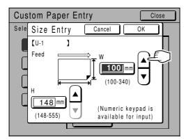
Facing towards the paper feeding direction (into Feed Tray), enter W (width) and H (height). Touch either [], or use Print Quantity Keys.
