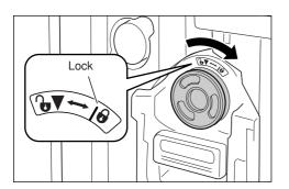
Turn the lnk Cartridge clockwise (  $\bigodot$  ) and lock in position.
