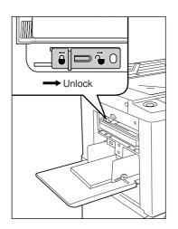
Grasp the Master Disposal Box handle and pull the box forward.
