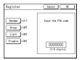
Up to 8 digits can be input. Press the  $\bigcirc$  key to clear the PIN code.
