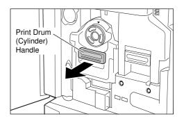
Grasp the Print Drum (Cylinder) Handle and slowly pull until the Print Drum (Cylinder) is completely extended.
