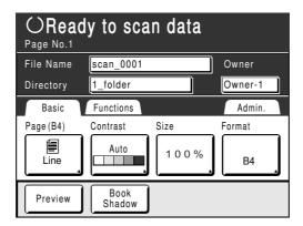
This setting is available when the optional Document Storage Card DM-128CF or USB Flash Drive is attached. The data in Storage Memory can be edited using Editor functions.
