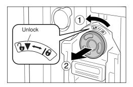
Turn the Ink Cartridge to the counter clockwise () and then pull it out.
