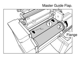
Insert the leading edge of the master into its entrance under the Master Guide Flap and advance it as far in as it will go ( $\bigcirc$ ). If the Master is loose, turn the flange at the right towards the rear and rewind ( $\bigcirc$ ).
