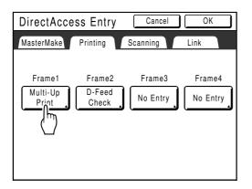
If the button has a function already assigned to it, the newly selected function will overwrite the previous function. **4** Select a function to assign.
