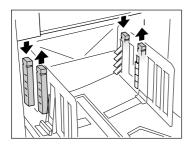
Press to open the two Paper Arrangers (right and left) closer to the machine.
