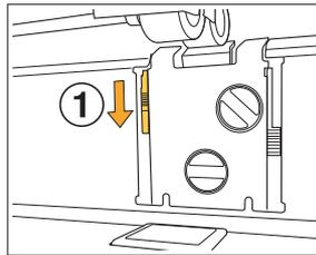
1 Lower the stripper lock knob (①) to unlock the stripper unit.
