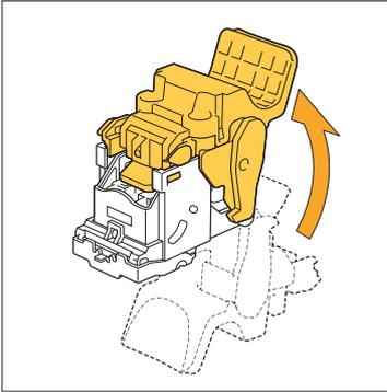
**9** Attach the cartridge to the unit while holding the cartridge handle.
