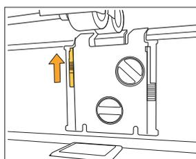
4 Lift the stripper lock knob to lock the stripper unit.
