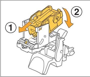
**!** • Align the projection on the front edge of the staple case with the staple cartridge.
