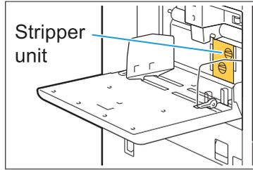
**Installing the stripper unit**
