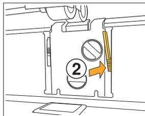
2 Press the stripper release lever (②) and remove the stripper unit.
