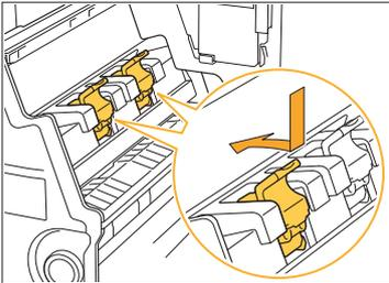
Align the ▲ marks on the cartridge and booklet unit when attaching the cartridge.
