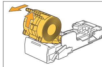
**4** Cut off the portion of the staples projecting to the outside of the staple case
