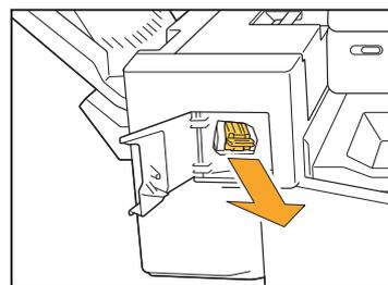
**3** Open the staple cartridge cover, and remove the jammed staple.
